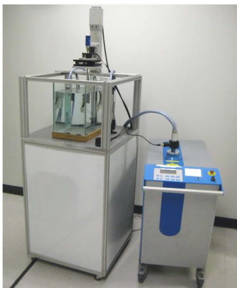
Fig. 3 – Setup of the mouse scanning system with rectangular fiber bundles.
