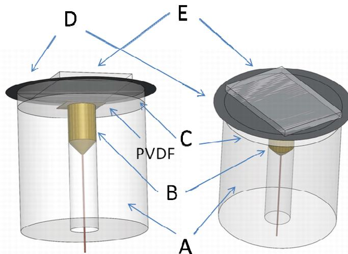
Figure 2. Experimental setup. A) acrylic body, B) brass backing used as signal electrical contact, C) light signal delay line (3 mm acrylic), D) light shield (metallized Mylar), and E) sample signal delay line (1.5 mm acrylic). Not shown is a 25 micron copper film, located between the square PVDF element and the light signal delay line, used as ground electrode. The entire body of the detector is also wrapped in copper foil (connected to ground) for electromagnetic shielding purposes.
