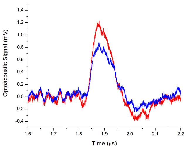
Figure 5. Optoacoustic signals collected from illumination of GNR adsorbed onto an acrylic substrate. Blank scans were subtracted in order to straighten the baseline, unfortunately also increasing experimental noise.
