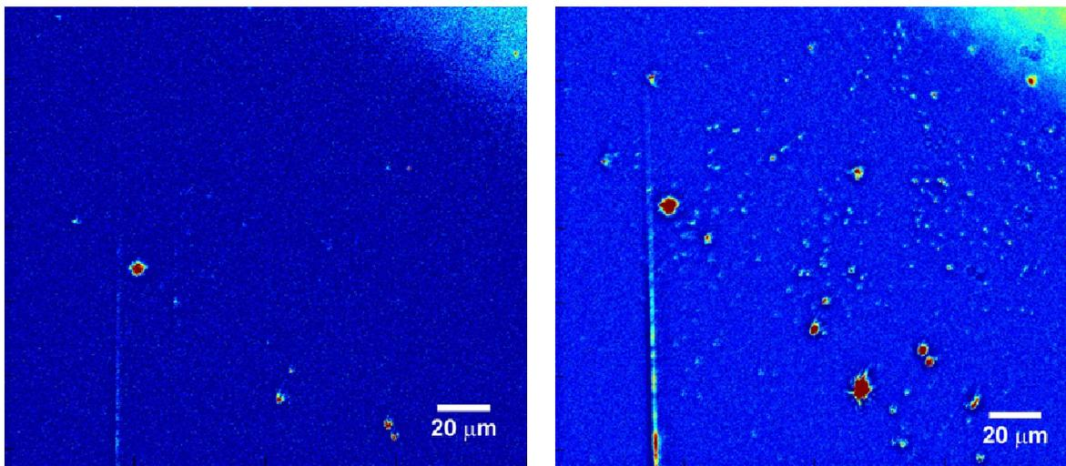
Figure 4. Dark field microscopy images of A) clean acrylic plate and B) acrylic plate coated with minute amount of heavily diluted pegylated GNR solution.
